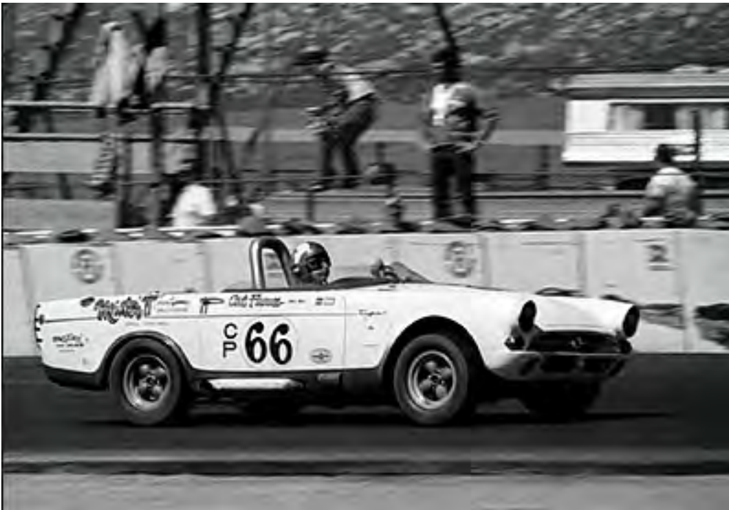
Art Firms at Riverside in 1968. Note that the side vents in the fenders are blocked and the LAT hood has been replaced by a stock steel hood. Photo: John Wilson
