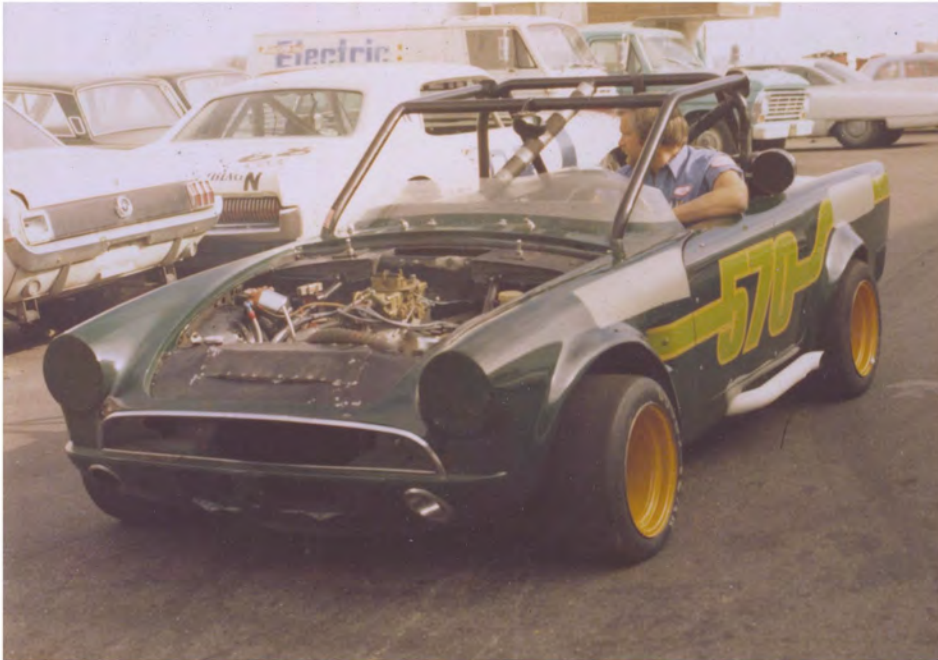
The Guldstrand Tiger in the paddock, after Gruys completed the body and paint work. Note the carbureted Wally Cartwright engine. The sponsorship credits to Cartwright and Preferred Rolls Services are covered by gray racing tape. 1980. Photo: Chris Gruys, 1980.
