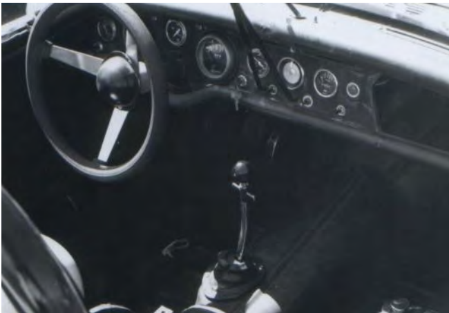
At Sears Point, the stock wood dash remains in the Tiger. An after-market tachometer has replaced the original Jaeger unit. 1971.
